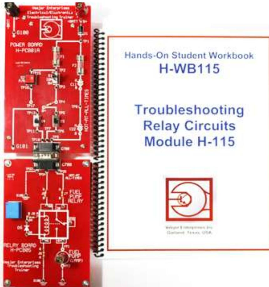
Relay Circuit Trainer H-PCB05 connects to the Power Board to complete the relay circuit for live relay circuit testing and troubleshooting.
